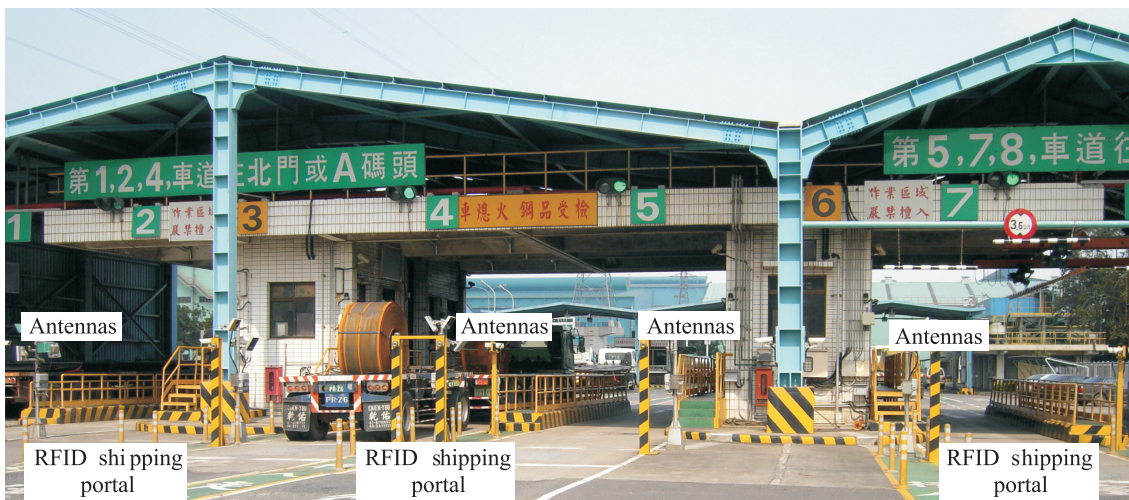
Fig.7. Panoramic view of the RFID multi-gate shipping portal.
